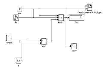
Fig 1: Simulink model of osmotic power & membrane flow
