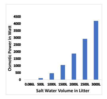
Fig. 9: Osmotic Power vs. Salt water volume
