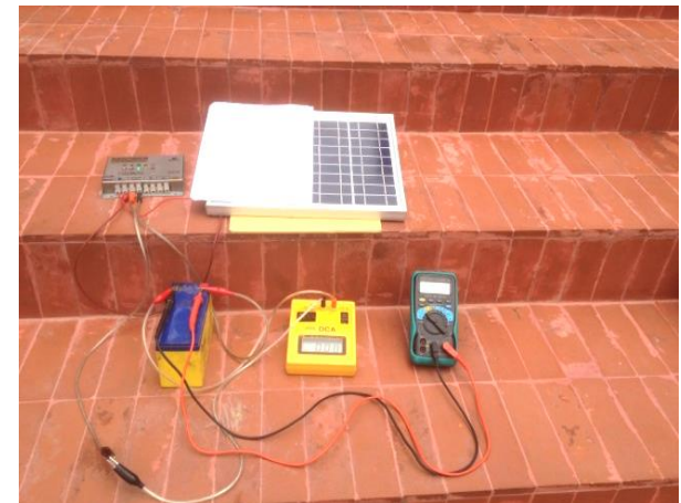
Fig. 9. Solar panel, DC Ammeter, Voltmeter, Battery, & Charge Controller used for data collection (with shading).
