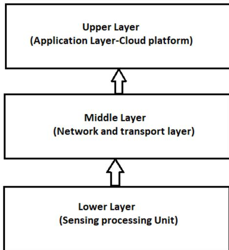
Figure 1. Three layer architecture of IoT
