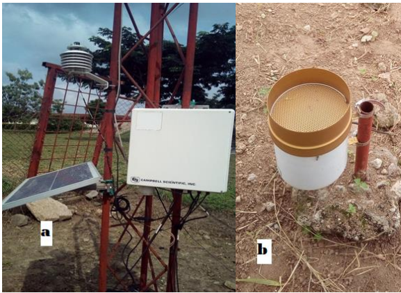
Figure 1. (a) The outdoor TRODAN measuring console equipped with a CR-1000 data acquisition system (b) The TRODAN in-situ measuring rain gauge
