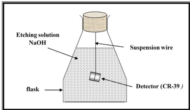
Figure 2. Chemical etching of the CR-39 track detector.
