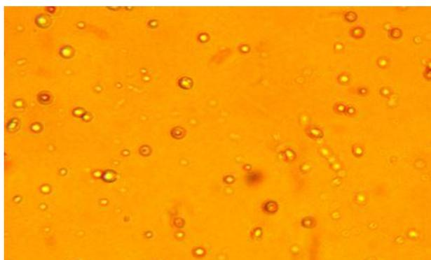
Figure 3. Tracks recorded on the CR-39 detector.
