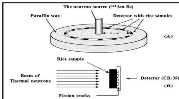
**Figure 1.** (A) The method of placing the studied and standard samples in paraffin wax in front of the neutron source. (B) The method of placing rice samples with the detector and recording the effects of fission tracks on the detector (Al-Bayati, 2019).
