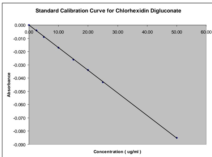
Figure 3. Standard calibration curve for chlorhexidine digluconate based on first-derivative spectrophotometry
