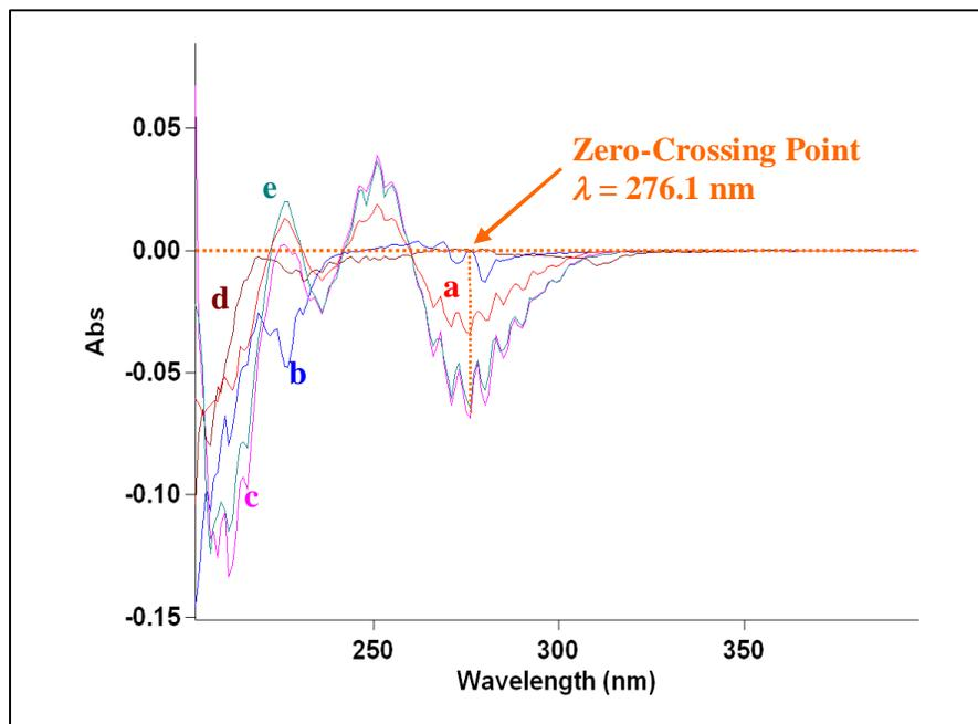
Figure 2. First-derivative spectra of (a) standard chlorhexidine digluconate solution, antimicrobial formulation (b) without chlorhexidine digluconate and (c) with chlorhexidine digluconate, dipped polymeric films' extracts (d) without chlorhexidine digluconate and (e) with chlorhexidine digluconate
