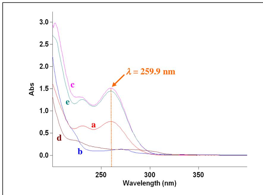
Figure 1. Zero-order spectra of (a) standard chlorhexidine digluconate solution, antimicrobial formulation (b) without chlorhexidine digluconate and (c) with chlorhexidine digluconate, dipped polymeric films' extracts (d) without chlorhexidine digluconate and (e) with chlorhexidine digluconate
