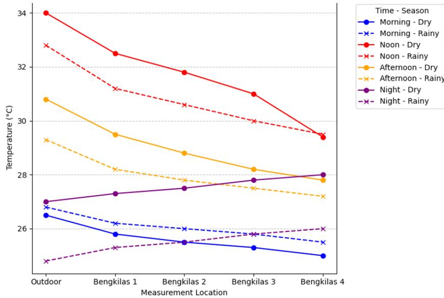
Figure 4. Temperature comparison across *bengkilas* tiers (example from a *Limas* house with four tiers).
