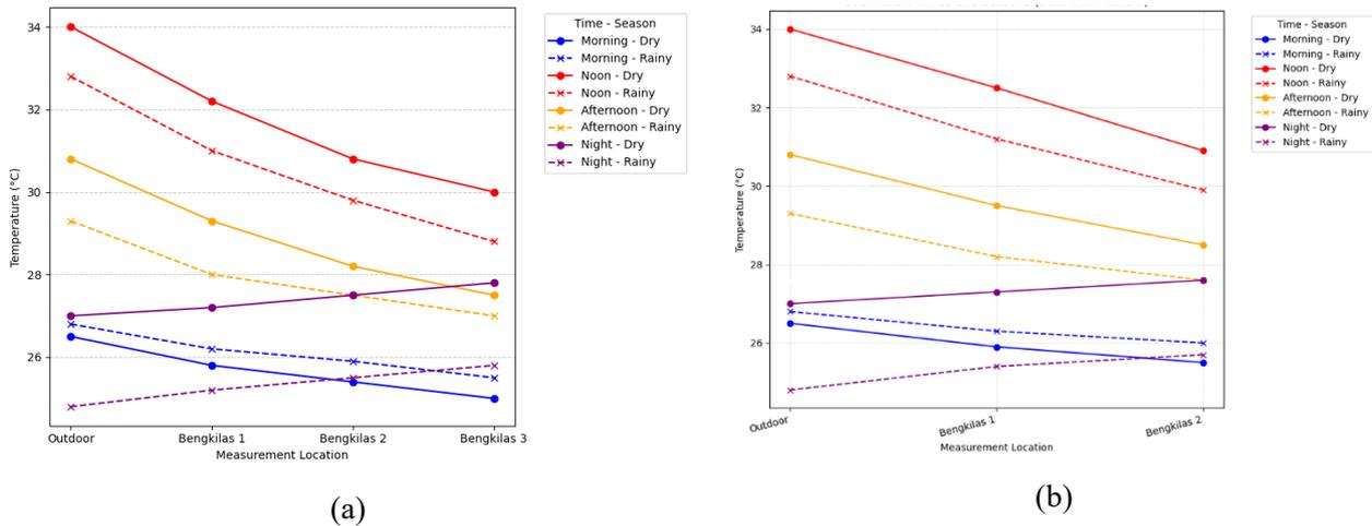
Figure 5. Temperature Comparison Across *Bengkilas* Tiers: (a) *Limas* House with Three *Bengkilas*; (b) *Limas* House with Two *Bengkilas*
