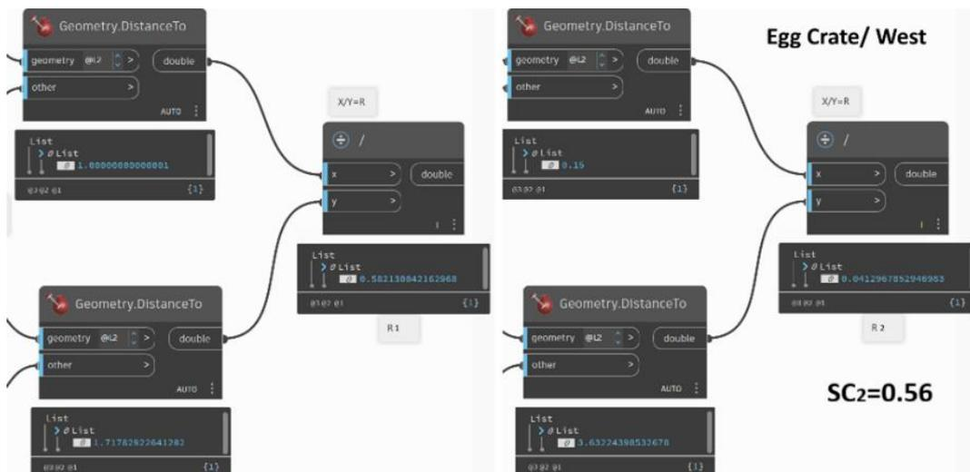
Figure 12. Calculating the SC<sub>2</sub> coefficient of egg crate projection
